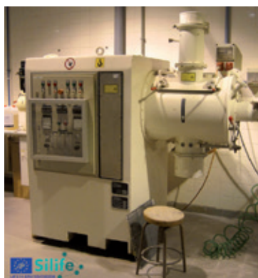
SILIFE PROJECT: PROTOTYPE DEVICE TO PRODUCE QUARTZ DUST BY USING COATING AGENTS
