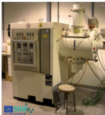
PROGETTO SILIFE: DISPOSITIVO PER LA COIBENTAZIONE DELLE POLVERI DI QUARZO CON COATING AGENTS
